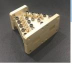
DPX-WC-22-28-34 is a WR34 diplexer with very wide bandwidth for both channels. Both channels provide 20% bandwidth with low insertion loss and low VSWR. Together, both channels cover nearly the entire WR34 waveguide band. It is very compact, nearly half the size of typical waveguide diplexers. Input and output are WR34 UG1530.
